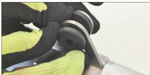
**ENG** Place the aluminum specers (3) on the silent-block washer (4) as shown in the picture and place them at the hole in the back side of the silencer support bracket. Place the silent block spacer (5) in the front side of the silencer support bracket at the hole.
