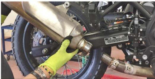
**ENG** Unscrew the screws to small metal clamp, the screw of the silencer support bracket and the remove the original exhaust.
