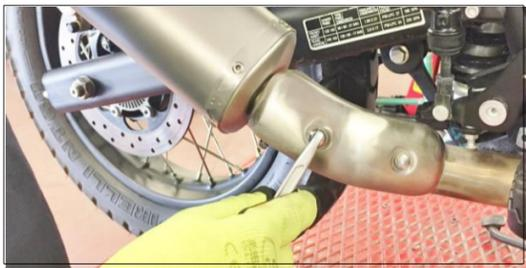
**ENG** Place the original heat shield and fix it using the original screw.
